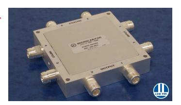
The 4x4 Hybrid is a matrix of four 3 dB Hybrid Couplers arranged so that signals applied to any of the four inputs will be split equally between the four outputs. This allows simple combining of multiple signals in the same wireless band to a common feeder cable, as might be required in a neutral host in-building distributed antenna system. Unused ports must be terminated externally in  $50\Omega$ .
